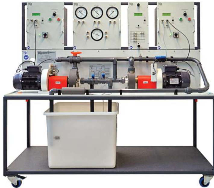
Figure 4: Experimental apparatus for pumps connection of TecQuipment [8]
